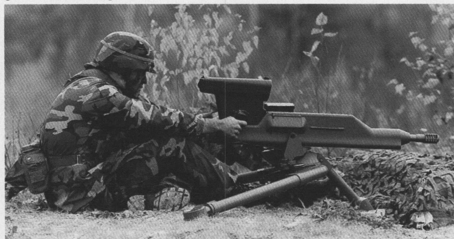
The bigger brother of the OICW is the OCSW or Objective Crew Served Weapon. It can fire 25-mm. exploding shells at a rate of 260 rounds per minute at a range of 2,000 meters. The weapon is being considered as a replacement for the MK19 grenade machine gun.
