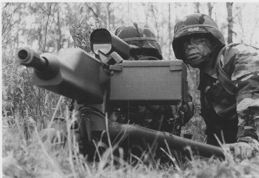
The bigger brother of the OICW is the OCSW or Objective Crew Served Weapon. It can fire 25-mm. exploding shells at a rate of 260 rounds per minute at a range of 2,000 meters. The weapon is being considered as a replacement for the MK19 grenade machine gun.
