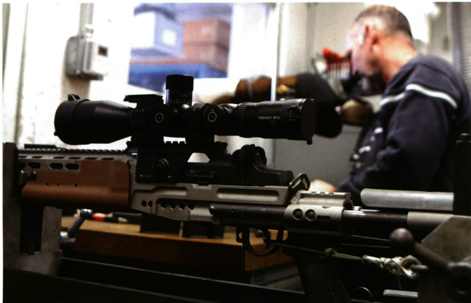
Kevin Kistler (above) fires a 7.62 mm M39 Enhanced Marksman Rifle from a test rack. The rifle will be fired at least 81 times and won't be sent to Marine marksmen until it passes PWS Marine specifications. Sgt Hamlet Tavarez (below left) is learning to become a precision weapons technician. It takes about a year of schooling. PWS leathernecks keep a record of every handmade weapon until the end of its service life when it comes back to PWS to be cut up and sold for scrap.
