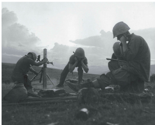
Mortars, with their high trajectory, proved invaluable in the often quick and close skirmishes. An 81 mm mortar crew with D/1/4 launches a 9-pound round with a bursting radius of 30-by-20 yards.
