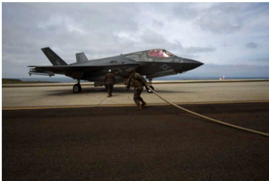
1 MEFLCpl Sebastian, a Bulk Fuel Specialist with Marine Wing Support Squadron 371, pulls a fuel nozzle to a Lockheed Martin F-35 Lightning II during jump forward arming and refueling point operations at advanced Naval Base San Clemente Island, CA, during Exercise PACIFIC BLITZ 19. (Photo by LCpl Tia Carr.)
