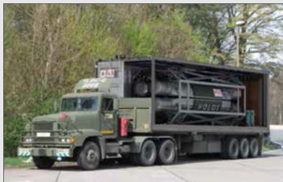
Figure 4. Holos micro reactor onboard a flatbed. The Holos microreactor can be scaled from a minimum of three MWe to a maximum of thirteen MWe for Holos Quad generators and comprised within a single transport container. The Air Force intends to field a similar prototype micro nuclear reactor at Eielson AFB, AK, by 2027 to allow that remote site to reduce reliance on
