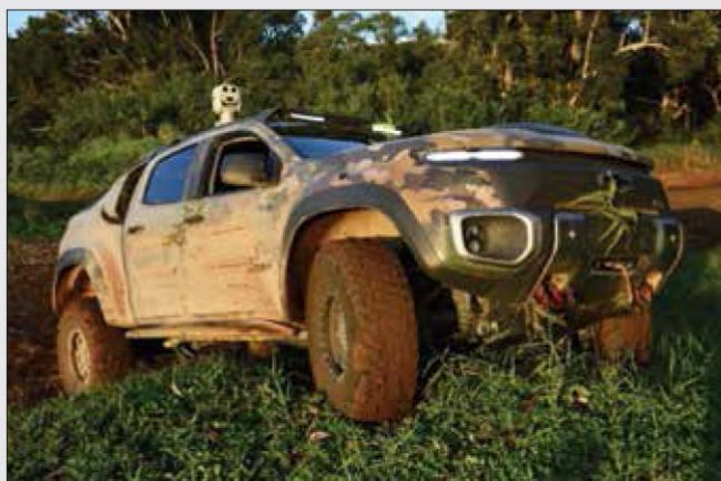
Figure 6. The ZH2 is a hydrogen-powered vehicle undergoing user evaluation in Hawaii with 25th Infantry Division. (Information available at https://www.army.mil ). (Figure provided by author.)
