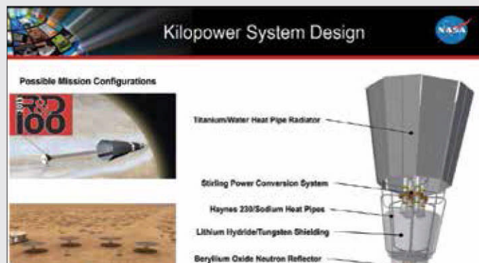
Figure 3. KRUSTY design and mission configuration. (Information available at: https://www.nasa.gov .) (Figure provided by author.)
